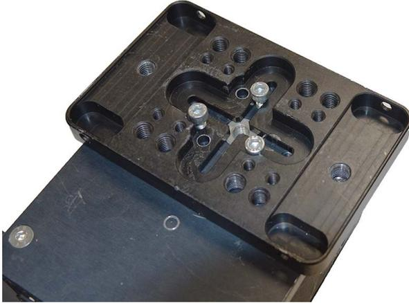
Add the 2x M10 washers between the scaffolding clamps and the mounting plate before securing the clamps using the 2x M10x20 screws.
