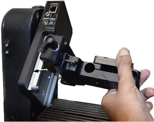
Once in position, tighten the knob screw to secure the tilt platform.
