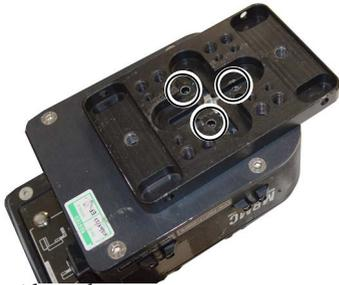
Align the 3x screw cavities in the head base and mounting plate and add 3x M6x12 screws
