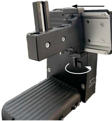
2. Loosen the knob in the roll assembly and add the roll assembly to tilt. Secure the roll assembly on tilt by tightening the knob.
