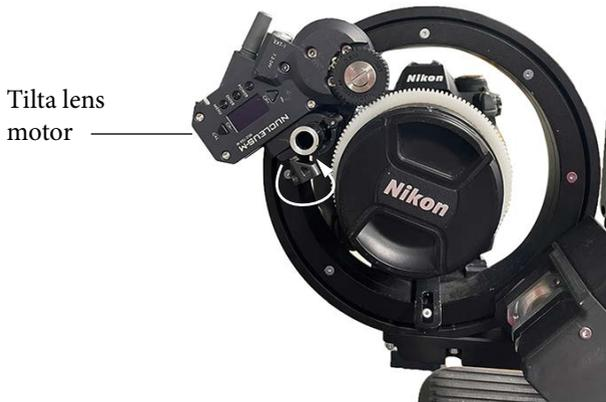
You can daisy-chain up to three Tilt motors. You can use any software, such as NXField or MHC, to control manual lenses and keyframe.
