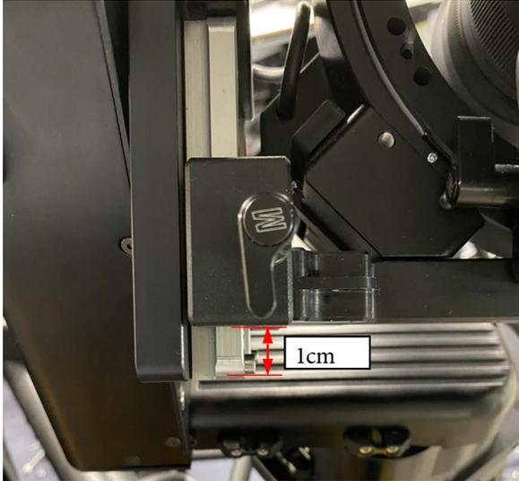
The recommended camera position is when the camera plate is moved all the way in and the camera screw in the following position:
