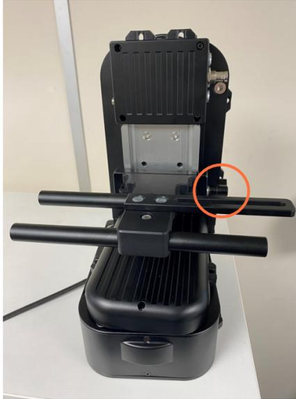
2. Fix the rods first before mounting the camera.
