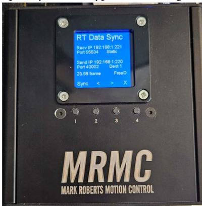
Flair would be configured to send to the Device's IP (default 192.168.1.221) and Port (default 55534). Do not use the "SYNC" mode of data export, use the default 50Hz output. The sync box currently supports Standard MRMC format Data, FreeD (Camera and Model Mover) as well as OSC format.
