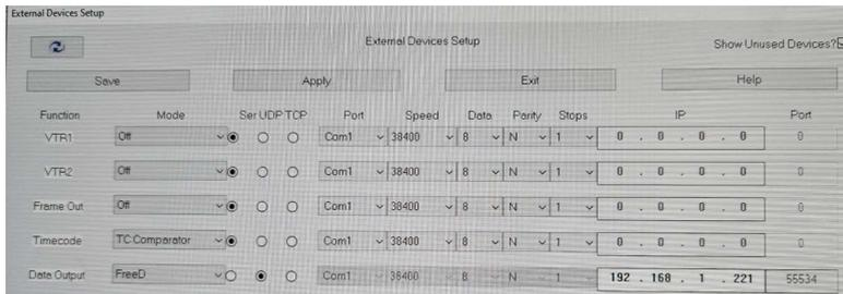
If the PC is connected to the network (This would be the INTIME network side of Flair that the RT unit and any axis boards are connected to) then the user should be able to log into the Configuration server on the sync box, simply by opening a browser and typing the IP address of the sync box (default of 192.168.1.221) into the address bar which presents the External Device setup screen.
