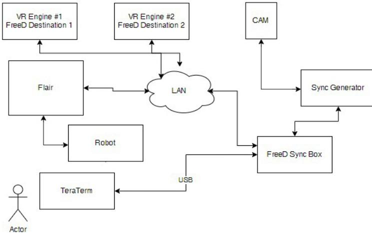
Connect the Flair Virtual Production Sync box to the same network as that of Flair PC. Power up the sync box by supplying 5VDC IN.
