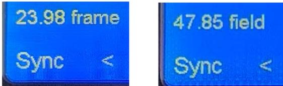
Holding the leftmost button for 5 seconds will switch between Send on Sync signal and Send on Data receipt. This is indicated by the frequency reading as “No Sync”
