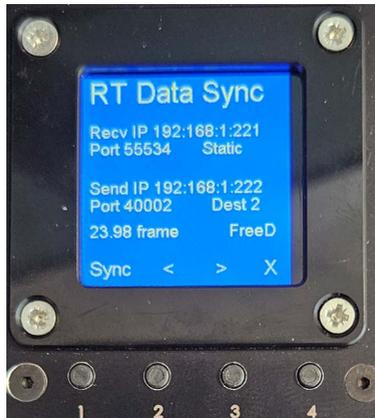
Holding down button 4 for 5 seconds will reset the device. This is useful to reacquire an IP from the DHCP server as the device will boot up faster than most Routers and would have chosen its default IP before the router booted.
