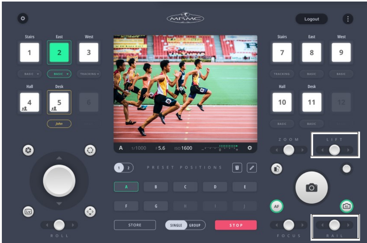
Example: Lift and Rail controls appearing for a head with 'child' rig type TRH.
